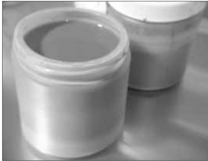
Settling and separation due to accelerated testing
