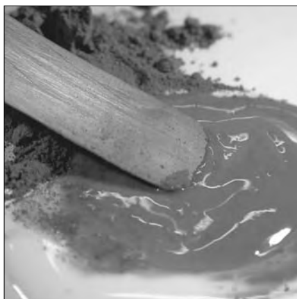
GAC 100 will wet out solids, including pigments, more readily than other polymers and is useful for artists formulating their own paints.
