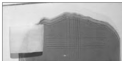
Pictured here are images after a "Tape Pull" glass adhesion test done in the GOLDEN Lab. GAC 200 (bottom) demonstrates its ability to adhere to nonporous surfaces such as glass.
