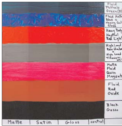
Test panel with rows of various colors and textures. One section was left untouched as a control. Other areas show affect of MSA Gloss, Satin, and Matte Varnishes applied over an isolation coat.
